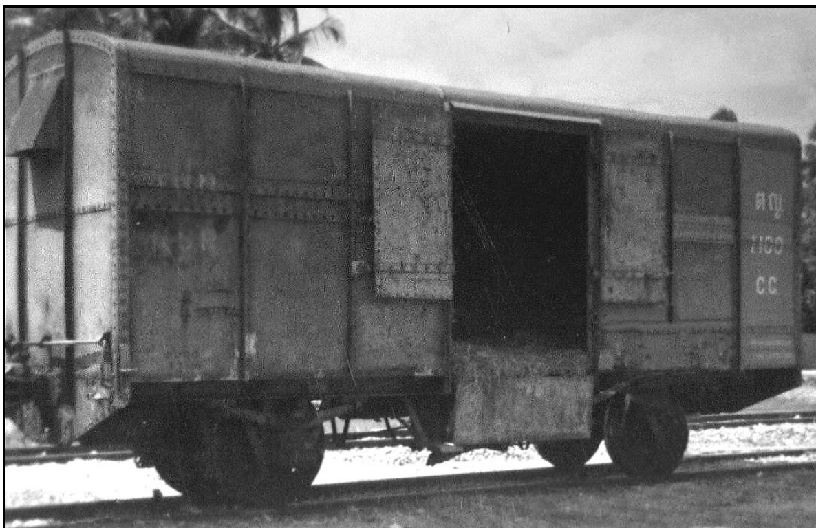
A TYPICAL STEEL SHEETED WAGON USED BY THE JAPANESE TO TRANSPORT THE POWs
